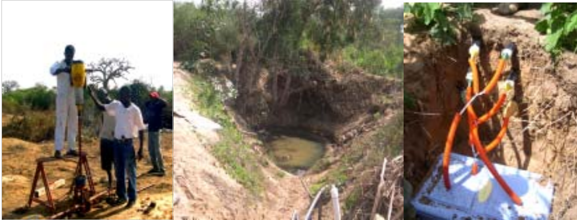
Fig3: water sampling. A) in piezometer (here under installation); B) in cèane; C) in lysimeter.
