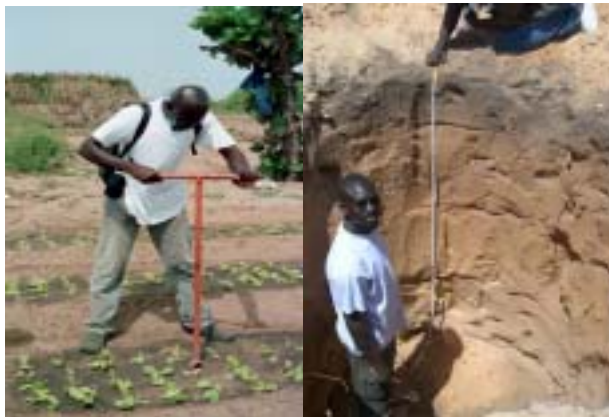
Fig2: soil sampling. A) with hand drill; B) in pedological pit.
