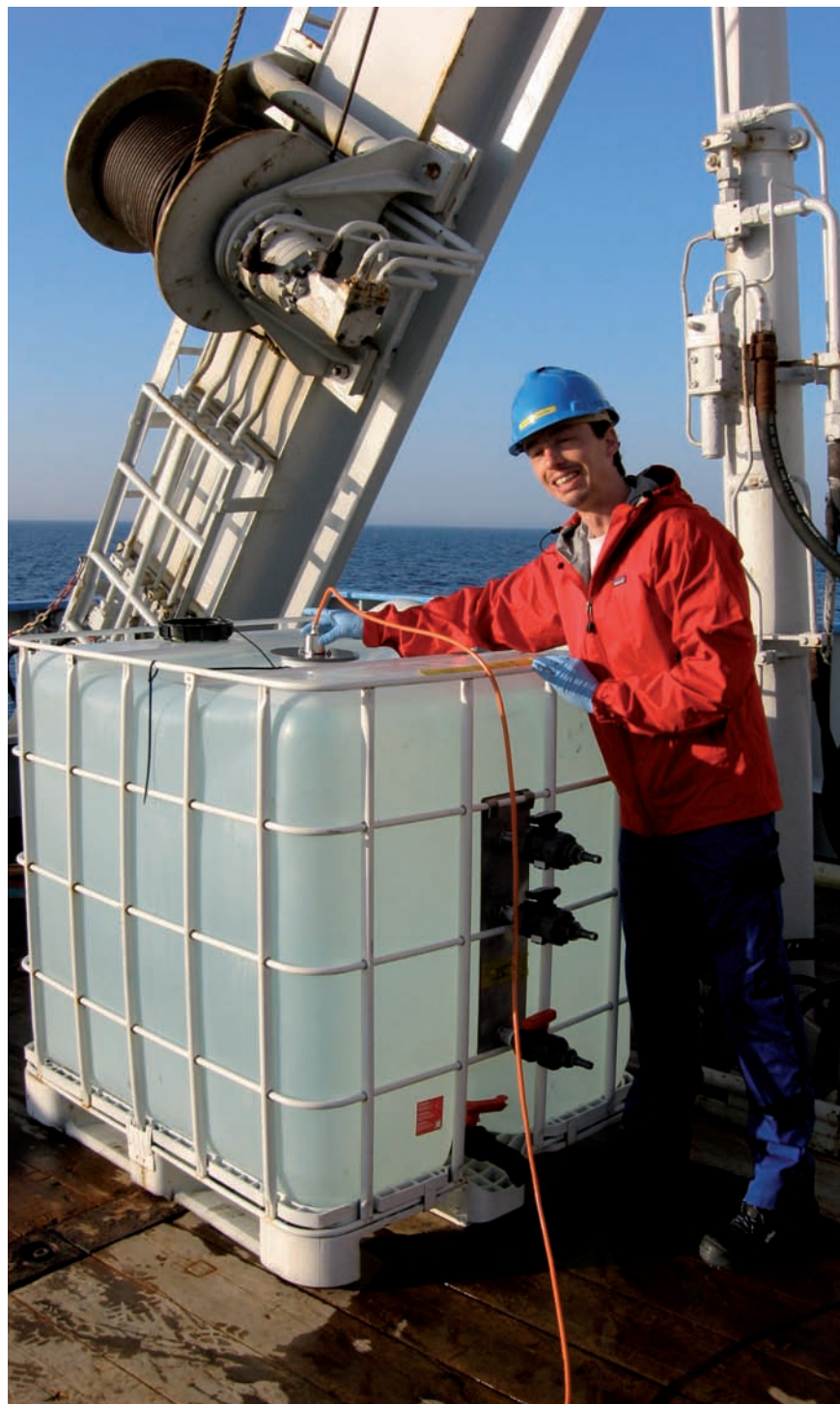
Getting the 1 cubic metre mesocosm vessels ready on board the RV Pelagia for a pilot oil spill
