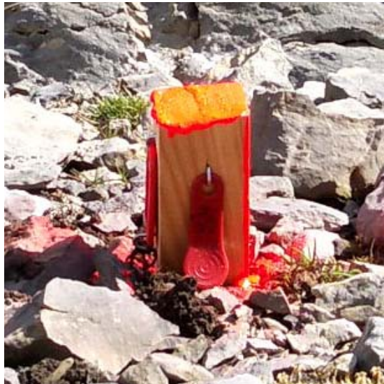
Figure 3 – Temperature logger, the cap of the surface logger is facing the South
