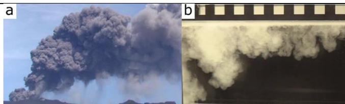
a) Image of ash fingers from the plume produced by the 2010 eruption of Eyjafjallajökull, Iceland. b) Analogue fingers created in the laboratory in experiments where a particle-bearing cloud (white) propagates above a denser ambient fluid (clear).
