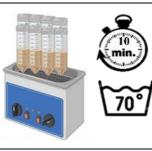
Immerse the tubes in the ultrasonic bath. Check the reaction after 10 min. If it reacts, extend the attack for 5 min and recheck. Close the tubes when finished.
