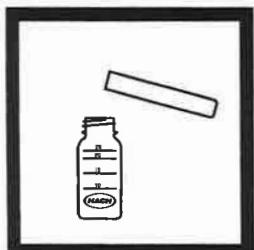
2. Pour the contents of the tube into the square mixing bottle.
