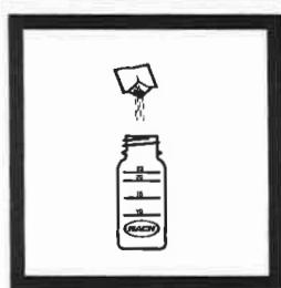
3. Add the contents of one Phenolphthalein Indicator Powder Pillow to the mixing bottle.
