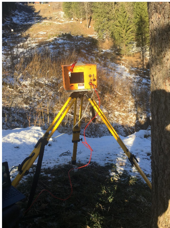
Figure 1 : Lidar measuring the main part of the landslide
