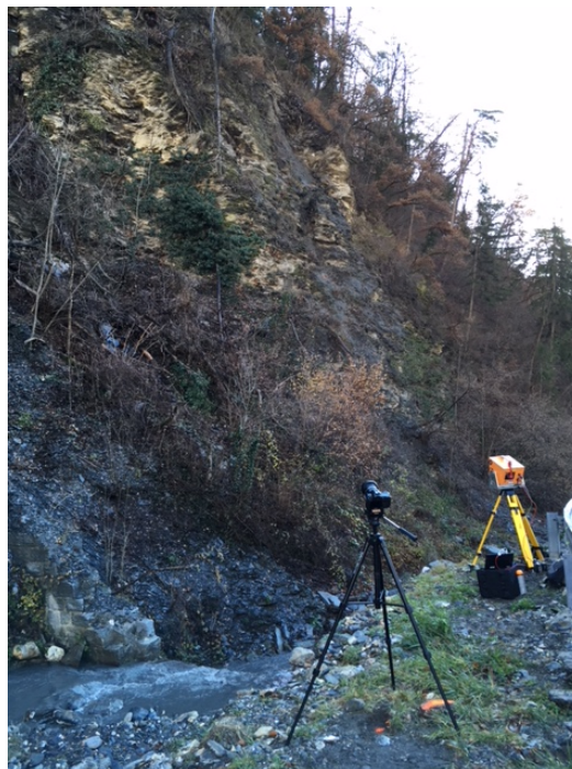
Figure 1: Field work illustrated by one slope movement near Sion, Valais. The two monitoring systems are used for comparison: acquisition by LiDAR and by camera.
