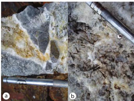
**Figure 3.** Breccia in N60°E trending vein. a) Different replacement intensities and quartz generations. b) Platy moulds possibly from platy-calcite related to late barren quartz, pretty typical (relict) boiling textures.
