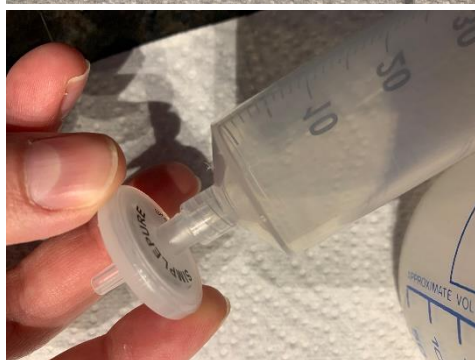
Attach the filter to the syringe by turning clockwise.
