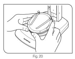
Place a specimen on the stage plate, hold the cup stage by the edge, and tilt the cup stage slowly. (Fig. 20)
