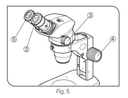
Eyepieces with eyepiece micrometer disk
